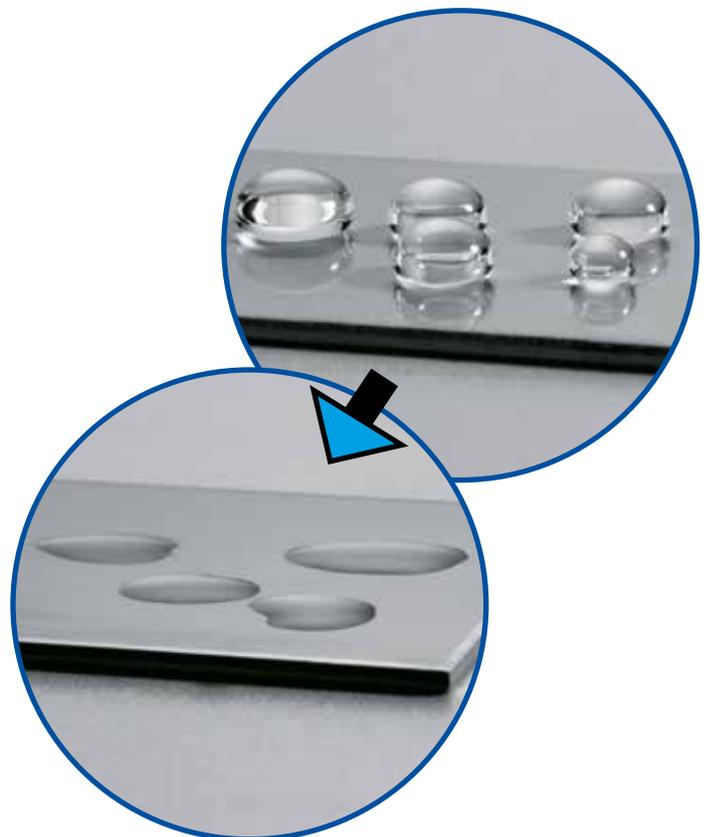
The cleanliness of the metal surface has also a great influence on the coating's adhesion. In their crude state, metals commonly used in the packaging industry are typically always covered with varyingly thick layers of oxides or anticorrosion products and protective oil. These impurities must be removed completely, if the proper coating wetting & adhesion strength is to be achieved.
